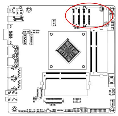
For example, the full size mSATA card that can be installed on a miniPCI express slot "MINI\_CARD1".
