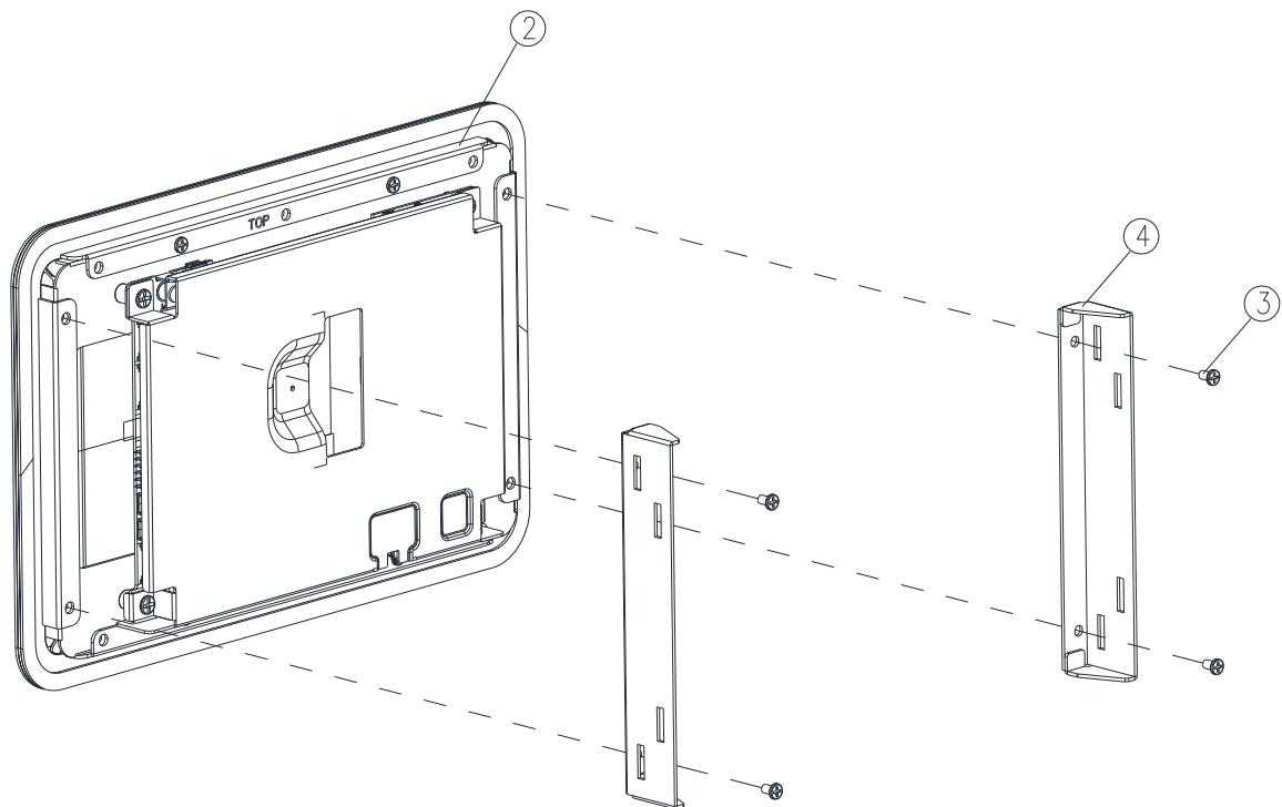
**Step2.** Insert and fasten 4 screws to secure Bracket R/L.
