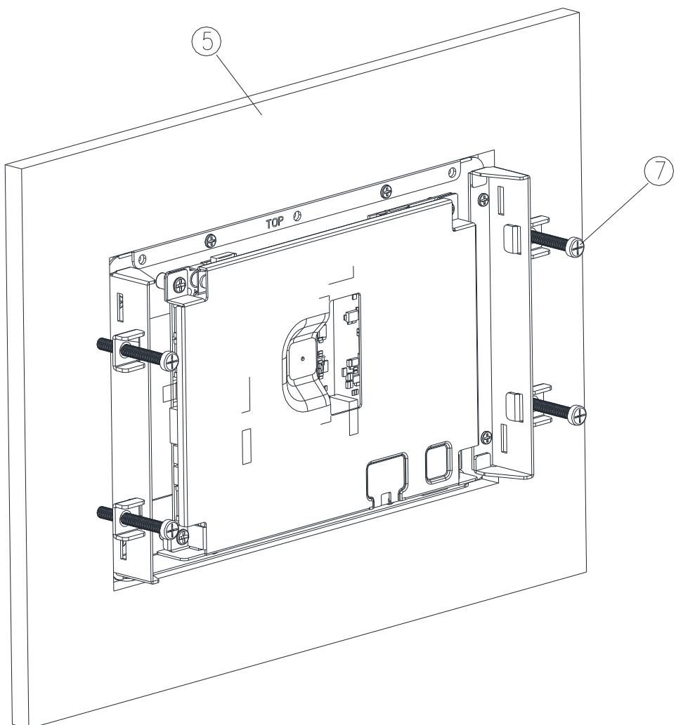
**Step5.** Insert and fasten 4 Panel mount screws to secure the module.
