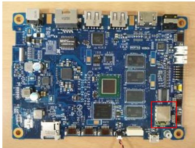
WiFi Module is located on MB underneath of the Shielding cover.
