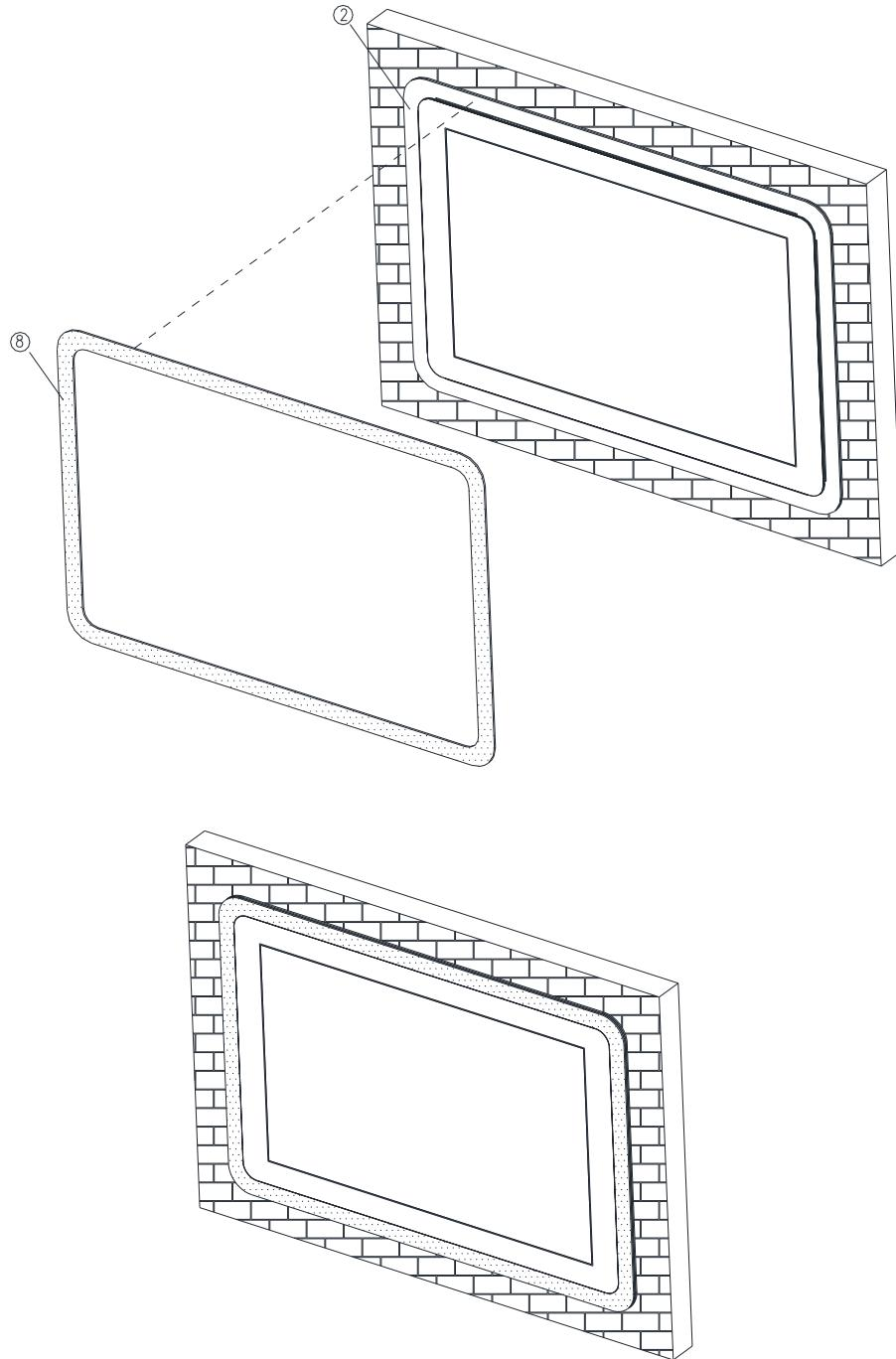
**Step6.** Paste the Decoration Plate on the Front bracket to complete installation.
