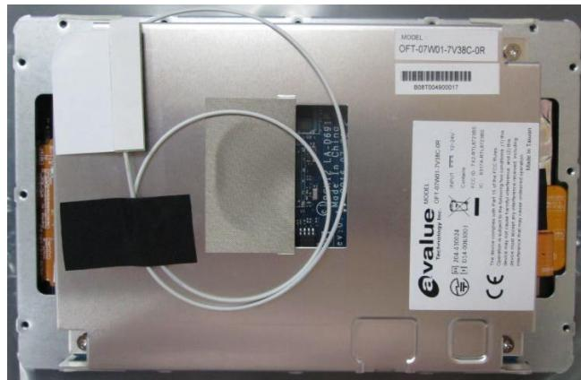
Remove all screws on shielding cover.
