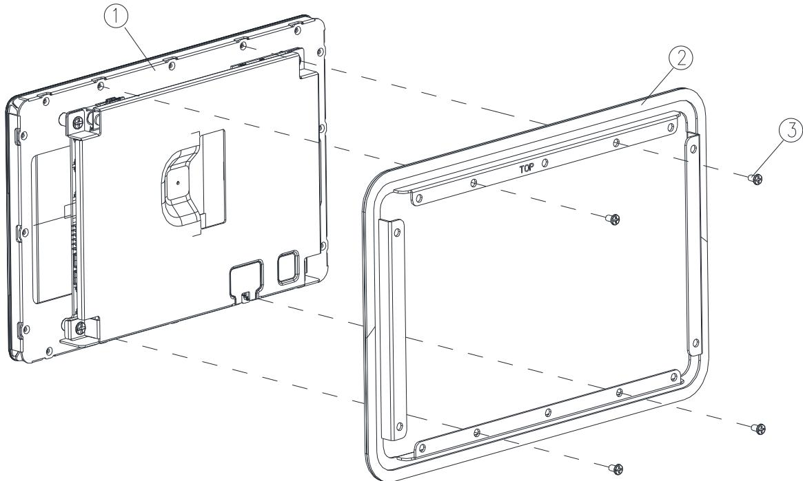
**Step1.** Insert and fasten 4 screws on each side of the monitor to secure Front bracket.
