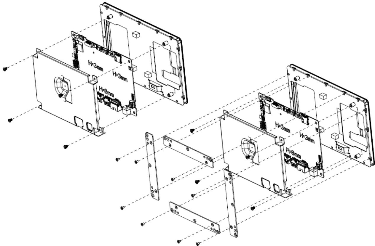
**Step1.** Locate brackets on both sides, matching the holes on the monitor.
