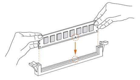
3. Firmly insert the DIMM into the socket until the retaining clips snap back in place and the DIMM is properly seated.
