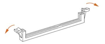
2. Align a DIMM on the socket such that the notch on the DIMM matches the break on the socket.
