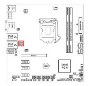
USB2\_PWR1 (For "USB2\_89" on rear I/O)
