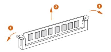
2. Remove the DIMM from the socket.
