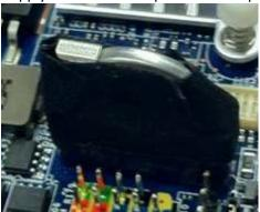
Apply heat shrink tubing on new production.
